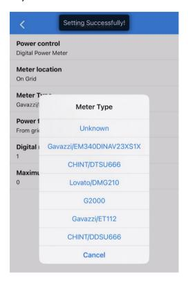
9. Power flow direction is by default 'rom grid to inverter'; Digital meter modbus address Is by default '1'. Set up the Maximum feed in grid power (export limit) as suggested by the local power distributor.
