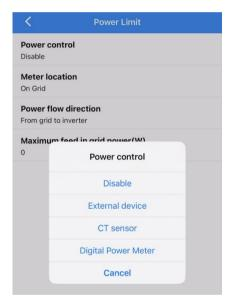
7. Meter location is usually 'On Grid' if you want to set up export limit and consumption monitoring
